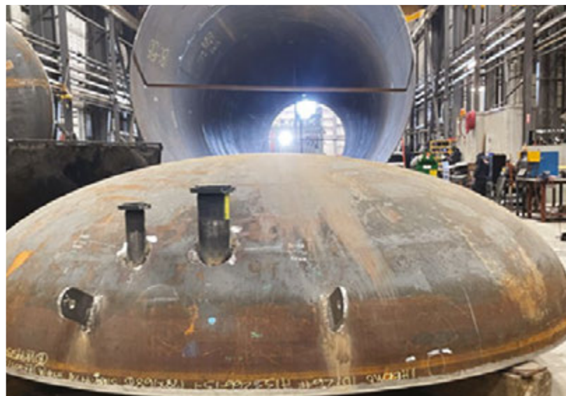
Treater vessel fabrication
